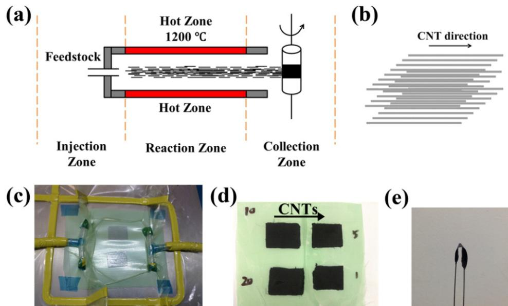
**Fig. 1.** Fabrication process of the CNT/epoxy films. (a) Schematic illustration of the fabrication of CNT plies by a FC-CVD method. (b) Schematic illustration of the arrangement of CNT plies. (c) Experimental set-up of the RTM process for preparing CNT/epoxy films. (d) As-prepared CNT/epoxy films with 1, 5, 10 and 20 CNT plies. (e) A flexible CNT/epoxy film bent by tweezers.
