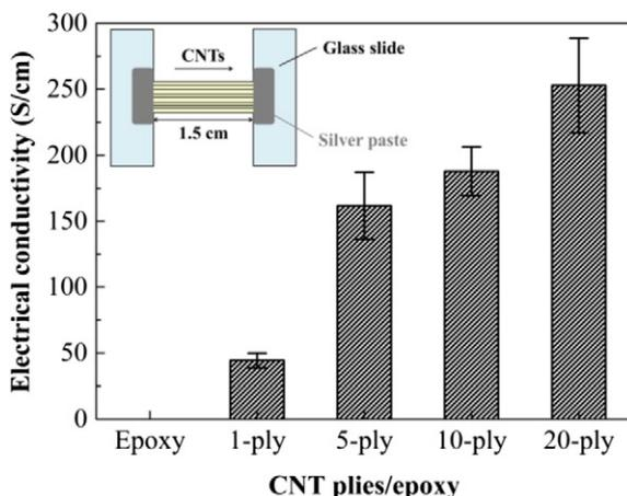
Fig. 8. Electrical conductivity of the CNT/epoxy films as a function of CNT plies.
