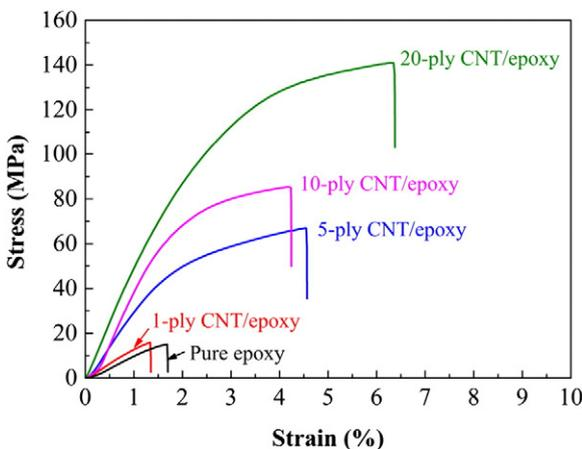
Fig. 5. Typical tensile stress–strain curves of CNT/epoxy films with different CNT plies.
