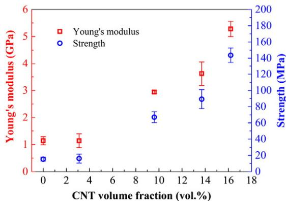
Fig. 7. Strength and Young's modulus of CNT/epoxy composite films as a function of CNT volume fraction.
