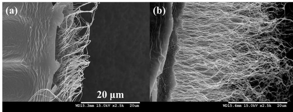
Fig. 6. SEM images of (a) 1-ply and (b) 20-ply CNT/epoxy composite films after tensile test.
