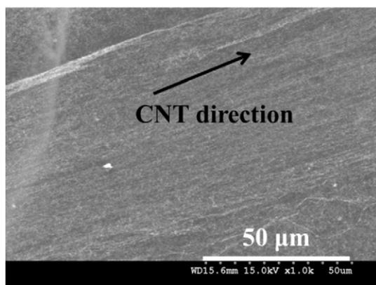
Fig. 2. An SEM image of the as-prepared CNT ply.
