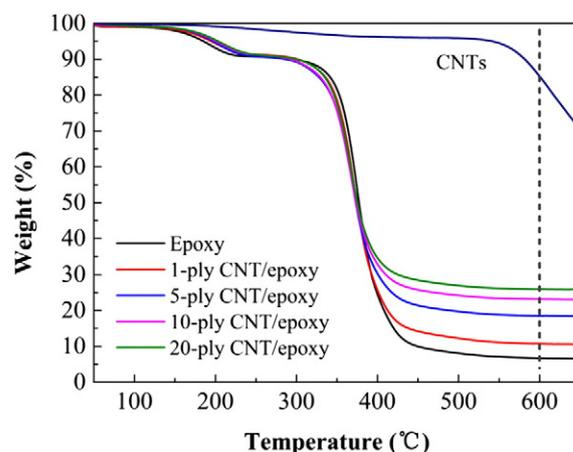
Fig. 3. TGA curves of pure CNT films, pure epoxy and CNT/epoxy films with 1, 5, 10 and 20 CNT plies.
