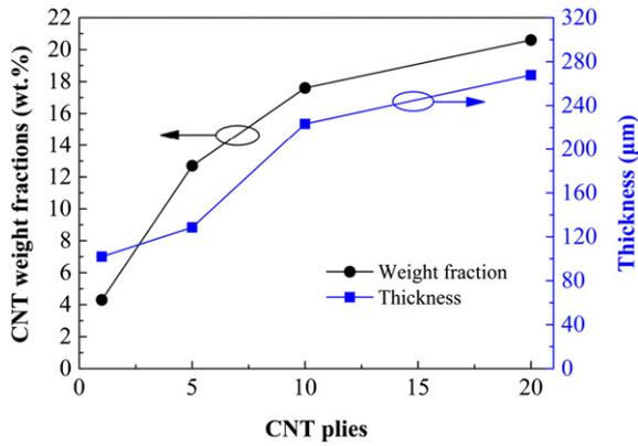
Fig. 4. The CNT weight fractions and the thickness of CNT/epoxy composite films as a function of CNT plies.
