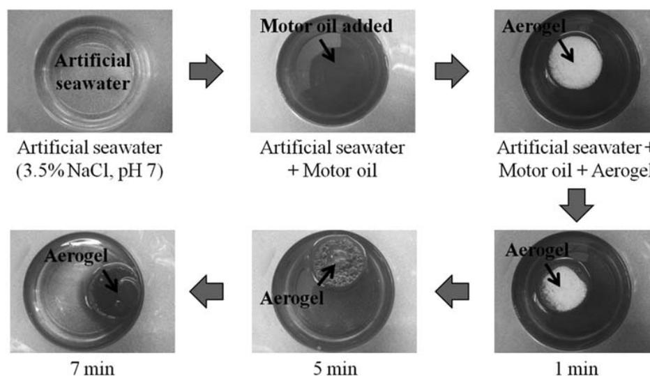
**Figure 14.5** Oil absorption process of the recycled cellulose aerogel with 0.5 wt.% of cellulose fibres in artificial seawater (3.5 wt.% NaCl and pH = 7) mixed with 5w40 motor oil and dyed with Sudan Red G before testing. (Reprinted from *Chemical Engineering Journal*, 270, J. Feng, S. T. Nguyen, Z. Fan, H. M. Duong, Advanced fabrication and oil absorption properties of superhydrophobic recycled cellulose aerogels, 168–175, Copyright 2015, with permission from Elsevier).
