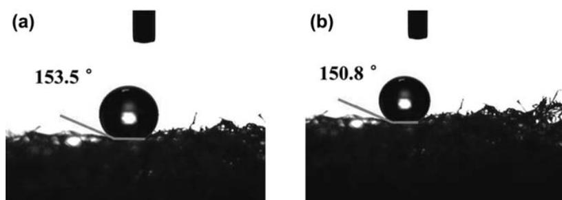
**Figure 14.3** Water contact angles on (a) the external surface and (b) the cross-section of the super-hydrophobic recycled cellulose aerogel.
