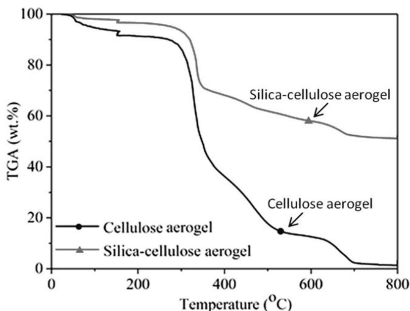
**Figure 14.10** The thermogravimetric analysis (TGA) curve of the silica–cellulose aerogel, compared with that of the cellulose aerogel using a Kymene binder. The composite aerogels were fabricated from cellulose matrixes with different cellulose fibre concentration of 4.0 wt.% in the initial suspensions.
