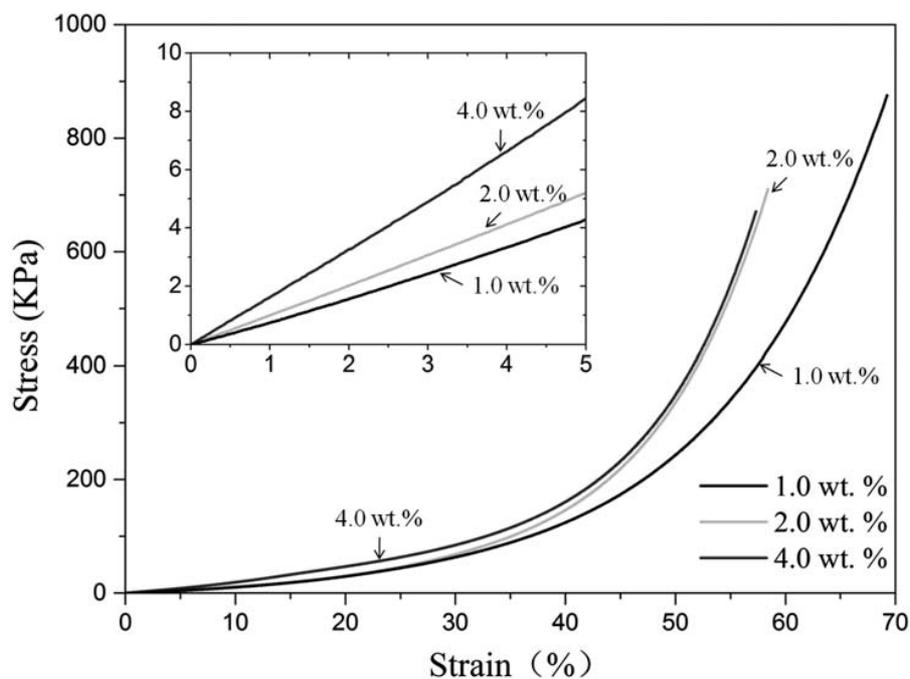
**Figure 14.11** The compressive strain-stress curves of the silica-cellulose aerogels fabricated from the cellulose matrixes with different cellulose fibre concentrations (1.0, 2.0, and 4.0 wt.%) in the initial suspensions. The magnified section shows the compressive curves at the low strain (up to 5%) for the composite aerogels.
