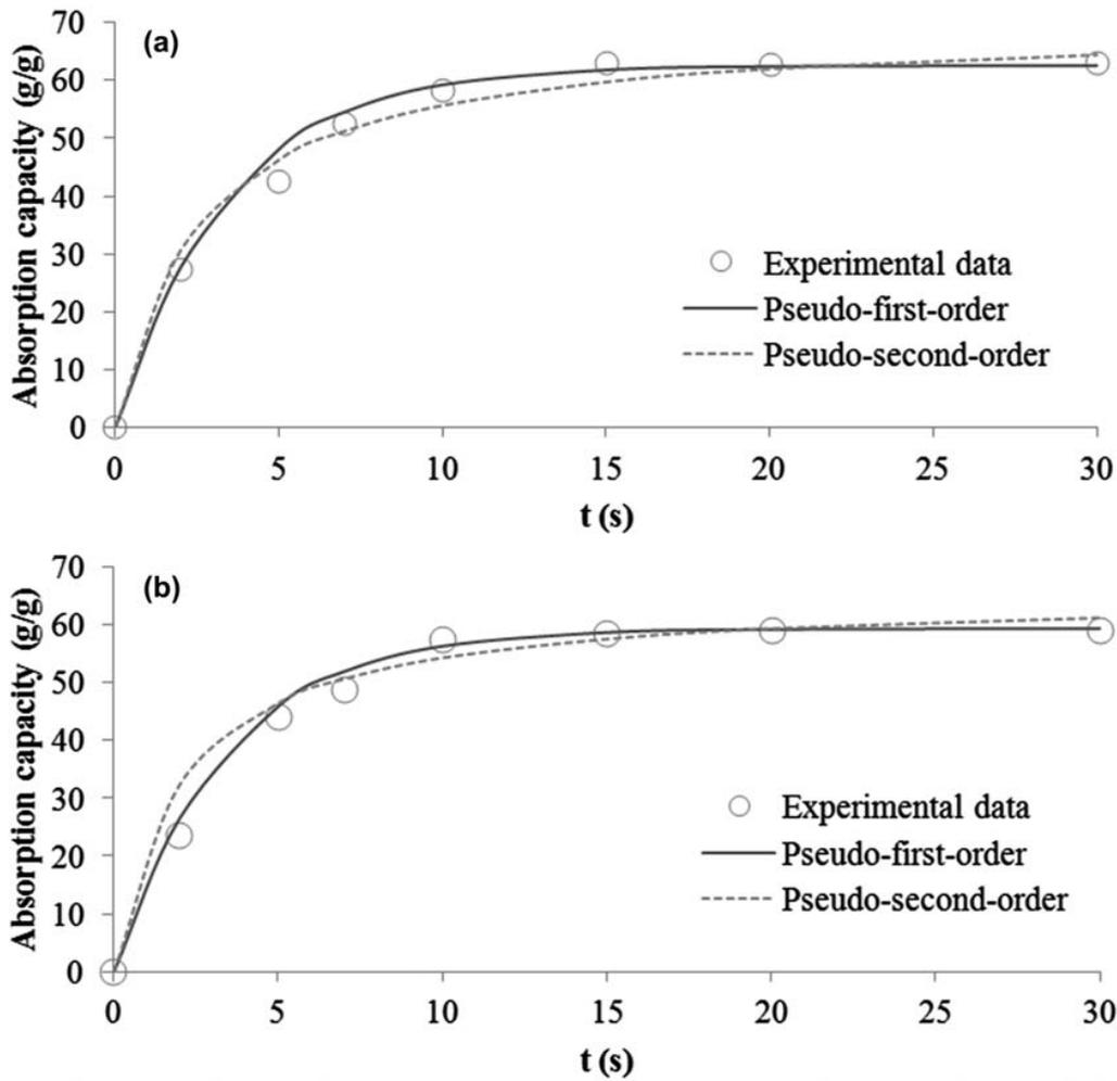
**Figure 14.7** Experimental data fitted with the pseudo-first-order and pseudo-second-order models for the absorption kinetics of (a) the 5w50 motor oil and (b) the Singer machine oil on the aerogel with 0.50 wt.% of cellulose fibres at 25 °C. (Reprinted from *Chemical Engineering Journal*, 270, J. Feng, S. T. Nguyen, Z. Fan, H. M. Duong, Advanced fabrication and oil absorption properties of superhydrophobic recycled cellulose aerogels, 168–175, Copyright 2015,with permission from Elsevier).
