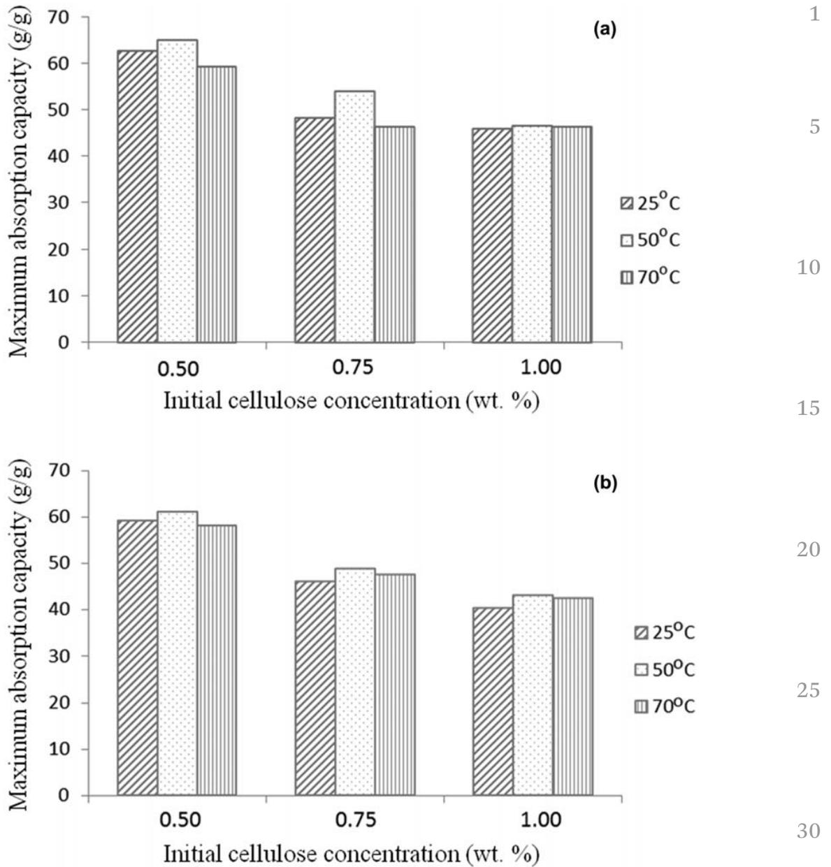
**Figure 14.4** Maximum absorption capacities,  $Q_m$ , of (a) the 5w50 motor oil and (b) the Singer machine oil with the recycled cellulose aerogels with various cellulose fibre concentrations of 0.50, 0.75, and 1.00 wt.% at 25, 50, and 70 °C.
