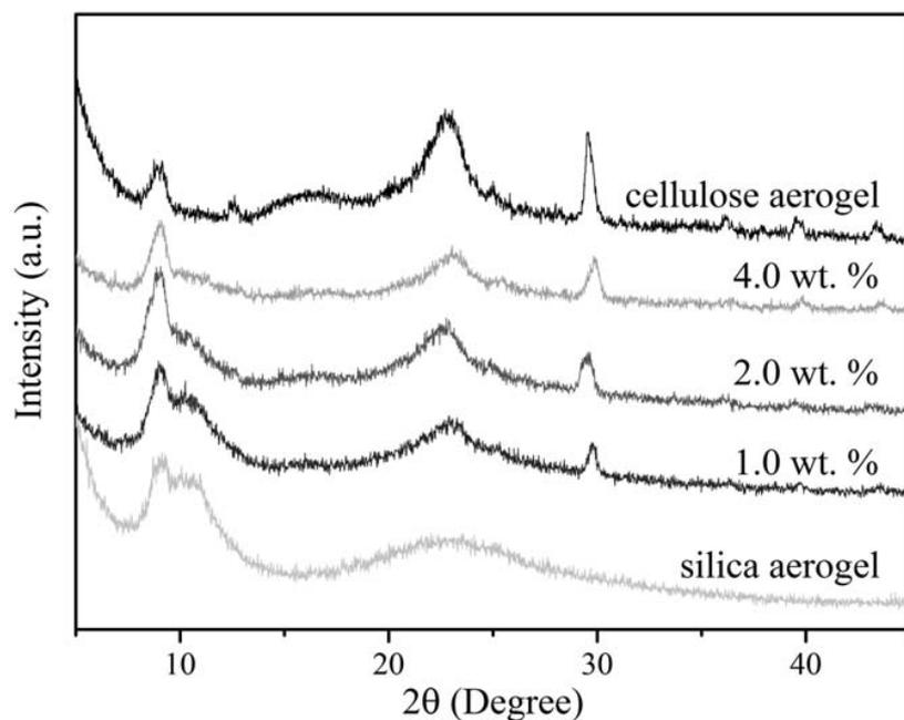
**Figure 14.9** XRD patterns of the silica aerogel, the cellulose aerogel, and the silica-cellulose aerogels fabricated from cellulose matrixes with different cellulose fibre concentrations (1.0, 2.0, and 4.0 wt.%) inside the initial suspensions.
