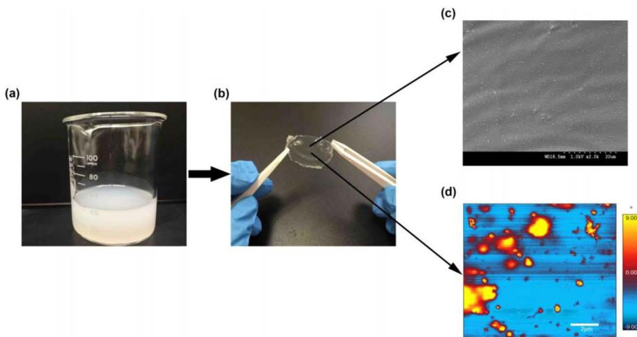
**Figure 1.** The PEO-immobilized ionogel: (a) A resin obtained from high energy ball milling. (b) Typical obtained ionogel membrane after solidifying. (c) SEM image of the ionogel membrane. (d) AFM phase image of the ionogel membrane.
