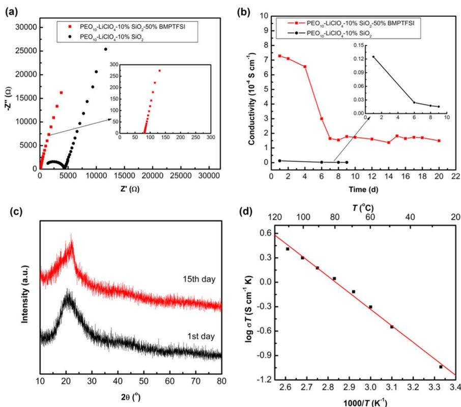
**Figure 2.** (a) The impedance plots of the as-prepared ionogel and polymer electrolyte without ionic liquid at room temperature. (b) The time evolution of room-temperature conductivities of the ionogel and polymer electrolyte without ionic liquid. (c) XRD patterns of the ionogel as prepared for 1 day and 15 days. (d) Arrhenius plot for the ionogel.
