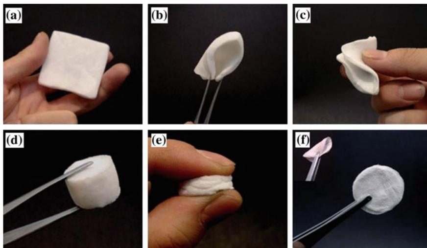
**Fig. 15.6** A demonstration of the flexibility and deformability of the aerogels. **a–c** The aerogel with dimensions of about  $5.44 \times 5.44 \times 0.59 \text{ cm}^3$  can be repeatedly bent as foldable as conventional paper. **d–f** Aerogel with a diameter of 2.10 cm and height of 1.67 cm can be compressed into a circuit sheet about 0.09 cm thick by hand; the obtained sheet can also be folded easily (Chen et al. 2011)
