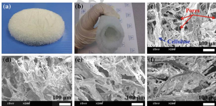
**Fig. 15.7** **a** Super-hydrophobic recycled cellulose aerogel, **b** flexibility of the large-scale cellulose aerogel ( $38 \times 38 \times 1$  cm) containing 0.60 wt% of the cellulose fibers, SEM images of the cellulose aerogels with different ratios of cellulose fibers (wt%) and kymene ( $\mu$ l): **c** 0.25:5, **d** 1.00:5, **e** 0.60:5 and **f** 0.60:20 (Feng et al. 2015)
