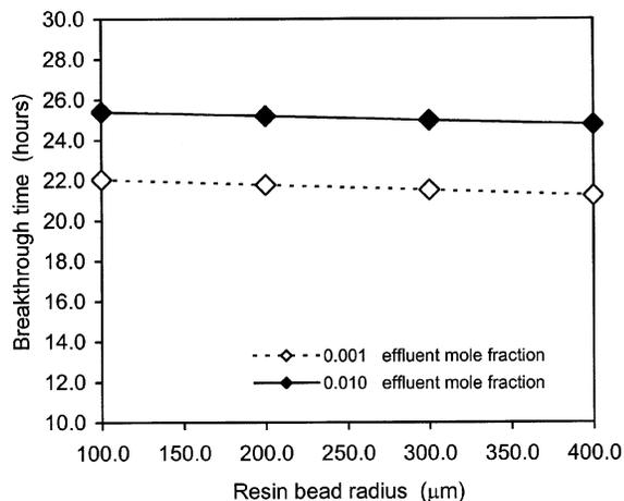
**Figure 10.** Effects of varying the resin bead sizes on the predicted ion exchange of the regeneration cycles as indicated by breakthrough times for an annular bed of the base case dimensions. Diverging flow.
