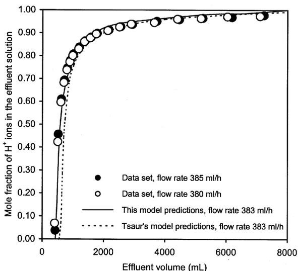
**Figure 4.** Breakthrough curve for the Ca-H regeneration runs using a 0.53 N HCl solution at a flow rate of 383 mL/h. Wedge-shaped cell resin bed initially in the Ca form.
