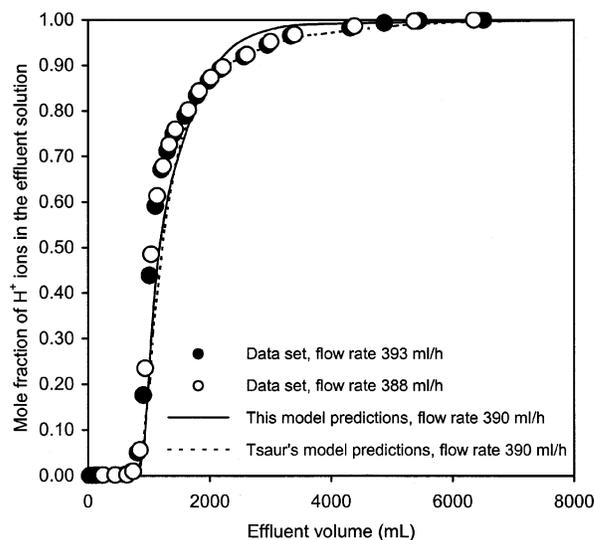
**Figure 2.** Breakthrough curves for the Na–H regeneration runs using a 0.53 N HCl solution at a flow rate of 390 mL/h. Wedge-shaped cell resin bed initially in the Na form.
