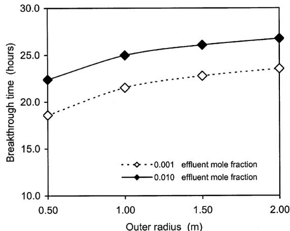
**Figure 8.** Predicted ion-exchange performance of the regeneration cycles as indicated by breakthrough times for an annular bed with  $R_o/R_i = 2.000$ . The bed height varies, and the bed volume remains constant. Diverging flow.
