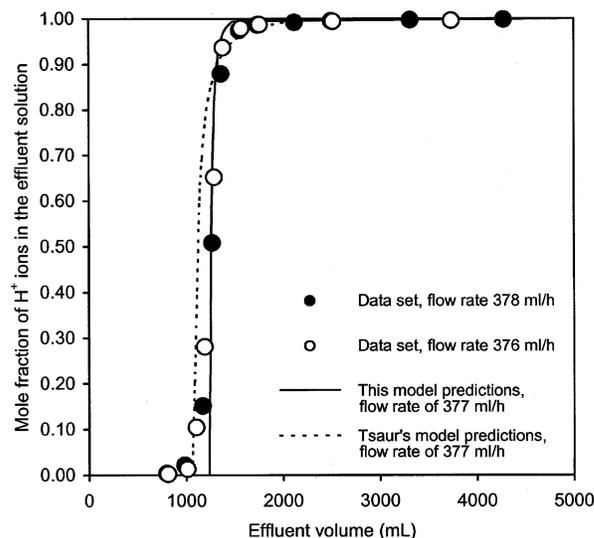
**Figure 5.** Breakthrough curve for the Ca-H exhaustion runs using a 0.50 N CaCl<sub>2</sub> solution at a flow rate of 377 mL/h. Wedge-shaped cell resin bed initially in the H form.
