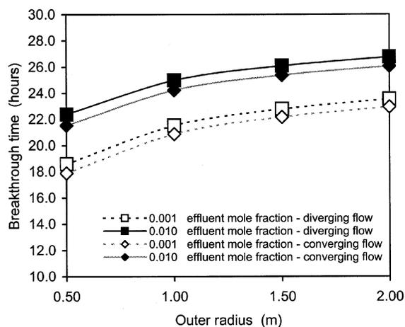
**Figure 13.** Effects of diverging and converging flow on the predicted ion-exchange performance of the regeneration cycles as indicated by breakthrough times for an annular bed with  $R_o/R_i = 2.000$ . The bed height varies, and the bed volume remains constant.
