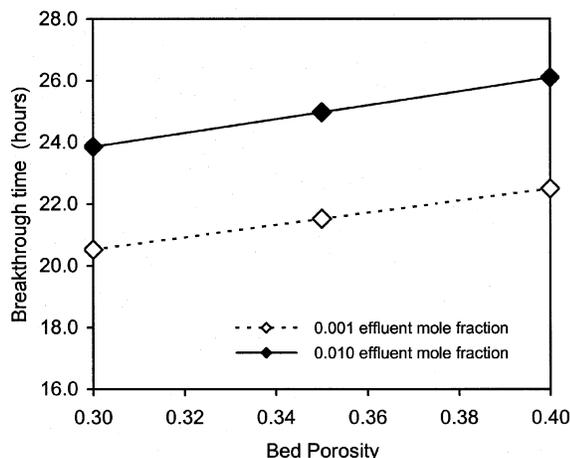
**Figure 6.** Effects of varying the bed porosity on the predicted ion-exchange performance of the regeneration cycles as indicated by breakthrough times for an annular bed of the base case dimensions. Diverging flow.
