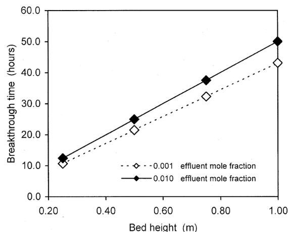
**Figure 9.** Predicted ion-exchange performance of the regeneration cycles as indicated by breakthrough times for an annular bed with  $H/V_{bed} = \text{constant}$ . The bed height varies. Diverging flow.
