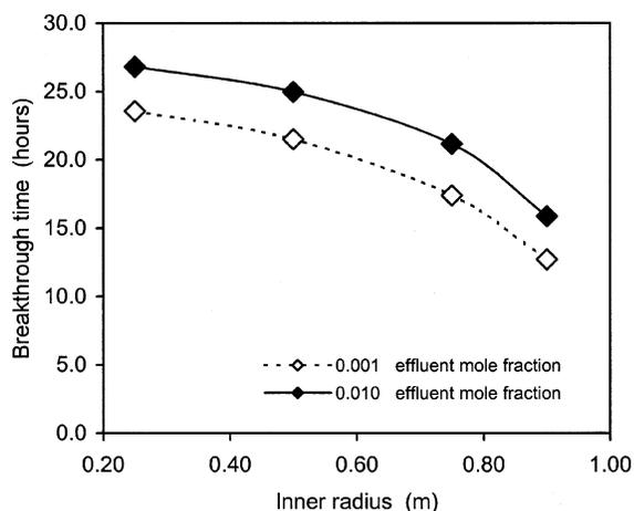
**Figure 7.** Predicted ion-exchange performance of the regeneration cycles as indicated by breakthrough times for an annular bed of a constant outer radius of 1.00 m but varying inner radius. The bed volume remains constant by varying the bed height. Diverging flow.
