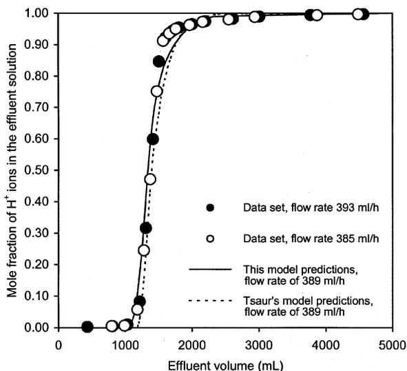
**Figure 3.** Breakthrough curves for the Na-H exhaustion runs using a 0.50 N NaCl solution at a flow rate of 389 mL/h. Wedge-shaped cell resin bed initially in the H form.
