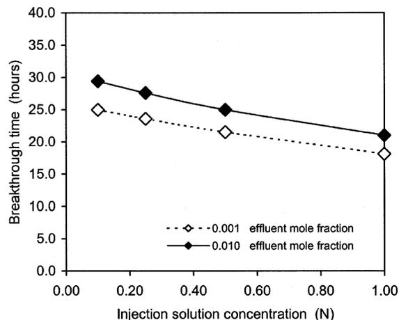
**Figure 12.** Effects of varying the injected solution concentrations on the predicted ion exchange of the regeneration cycles as indicated by breakthrough times for an annular bed of the base case dimensions. Diverging flow.
