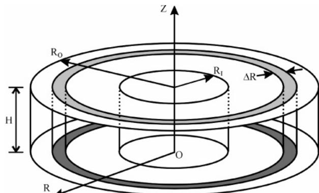
**Figure 1.** Representation of a fixed annular ion-exchange bed of constant thickness,  $H$ , showing the annular element.
