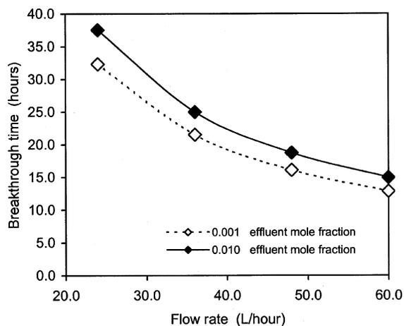
**Figure 11.** Effects of varying the flow rates on the predicted ion exchange of the regeneration cycles as indicated by breakthrough times for an annular bed of the base case dimensions. Diverging flow.
