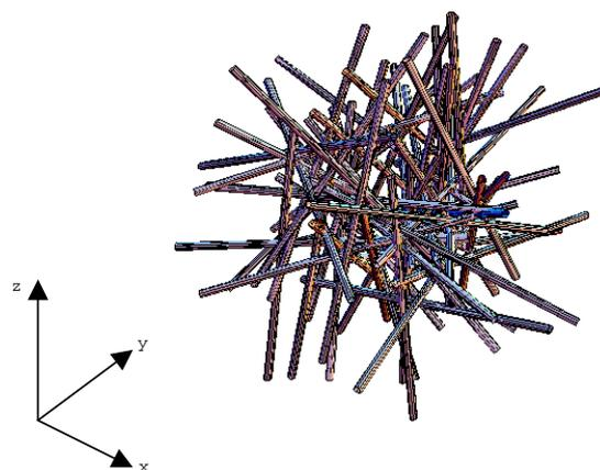
**Figure 5.** A model of SWNT composite material. The composite shown here is a realization of the case of disordered SWNTs at a weight fraction 0.10% and  $L/D = 40.0$ .
