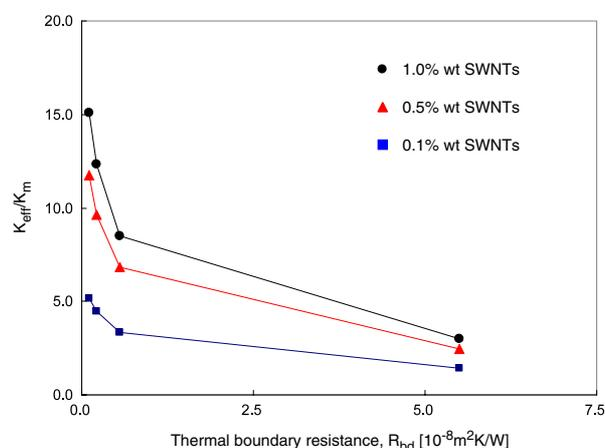
**Figure 6.** Effective thermal conductivity of SWNT-PMMA composites with SWNTs oriented parallel to the heat flux as a function of thermal boundary resistance with different weight fraction of SWNTs. For each value of thermal boundary resistance and weight fraction of SWNTs, the thermal conductivity is the average of three simulations with different initial SWNT distributions.
