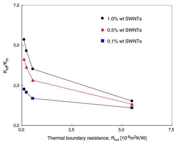
**Figure 7.** Effective thermal conductivity of randomly dispersed SWNT-PMMA composites as a function of thermal boundary resistance with different weight fraction of SWNTs. For each value of thermal boundary resistance and weight fraction of SWNTs, the thermal conductivity is the average of three simulations with different initial SWNT distributions.
