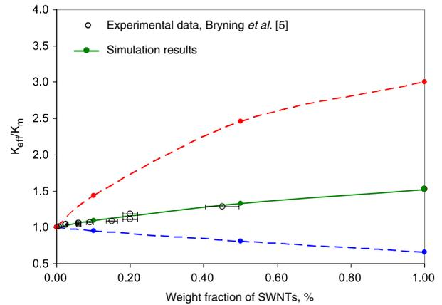
**Figure 3.** Validation of the computational model with comparison to experimental data for SWNT-epoxy composites. The upper and lower dashed curves indicate the potential maximum and minimum thermal conductivity, respectively. Dots on the dashed curves indicate the simulation results. The best fit line to the data (solid line) yields an  $f_{m-CN}$  consistent with physical data.
