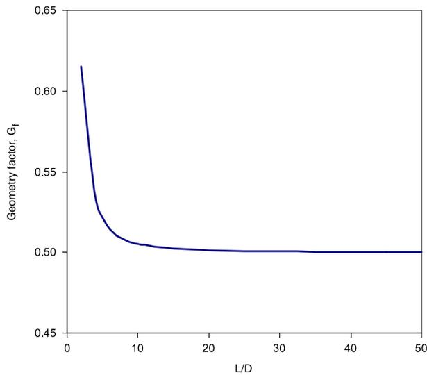
**Figure 1.** Effect of the aspect ratio  $L/D$  on the geometry factor.
