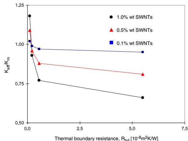
**Figure 8.** Effective thermal conductivity of SWNT-PMMA composites with SWNTs oriented perpendicular to the heat flux as a function of thermal boundary resistance with different weight fraction of SWNTs. For each value of thermal boundary resistance and weight fraction of SWNTs, the thermal conductivity is the average of three simulations with different initial SWNT distributions.
