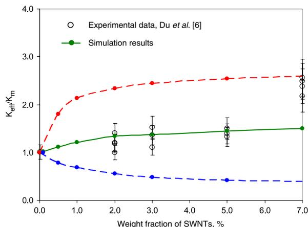
**Figure 4.** Validation of the computational model with comparison to experimental data of SWNT-PMMA composites. The upper and lower dashed curves indicate the potential maximum and minimum thermal conductivity, respectively. Dots on the dashed curves indicate the simulation results. The best fit line to the data (solid line) yields an  $f_{m-CN}$  consistent with physical data.
