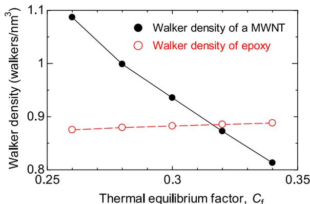
**Figure 2.** Average walker density of a MWNT (8.0 nm diameter, 300 nm length, 288 grid units) and epoxy with varied thermal equilibrium factor. The value  $C_f = 0.315$ , where the walker density inside and outside the CNTs is the same, is used in the MWNT in the simulations.
