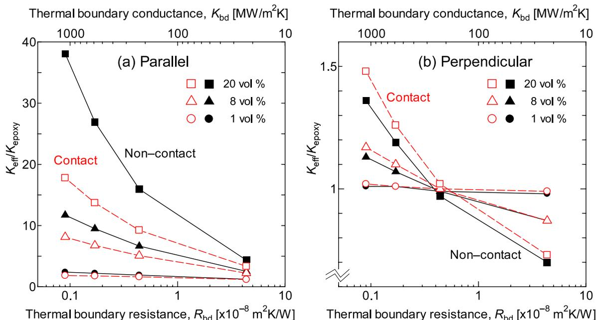
**Figure 3.** Effective thermal conductivity of MWNT-epoxy composites with MWNTs oriented (a) parallel and (b) perpendicular to the heat flux without (solid dots) and with (open dots) the inter-MWNT contact as a function of thermal boundary resistance with different volume fraction of MWNTs.
