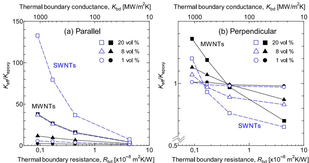
**Figure 5.** Comparison of effective thermal conductivity of MWNT-epoxy (solid dots) and SWNT-epoxy (open dots) composites with CNTs oriented (a) parallel and (b) perpendicular to the heat flux without the inter-CNT contact as a function of thermal boundary resistance with different volume fraction of CNTs.
