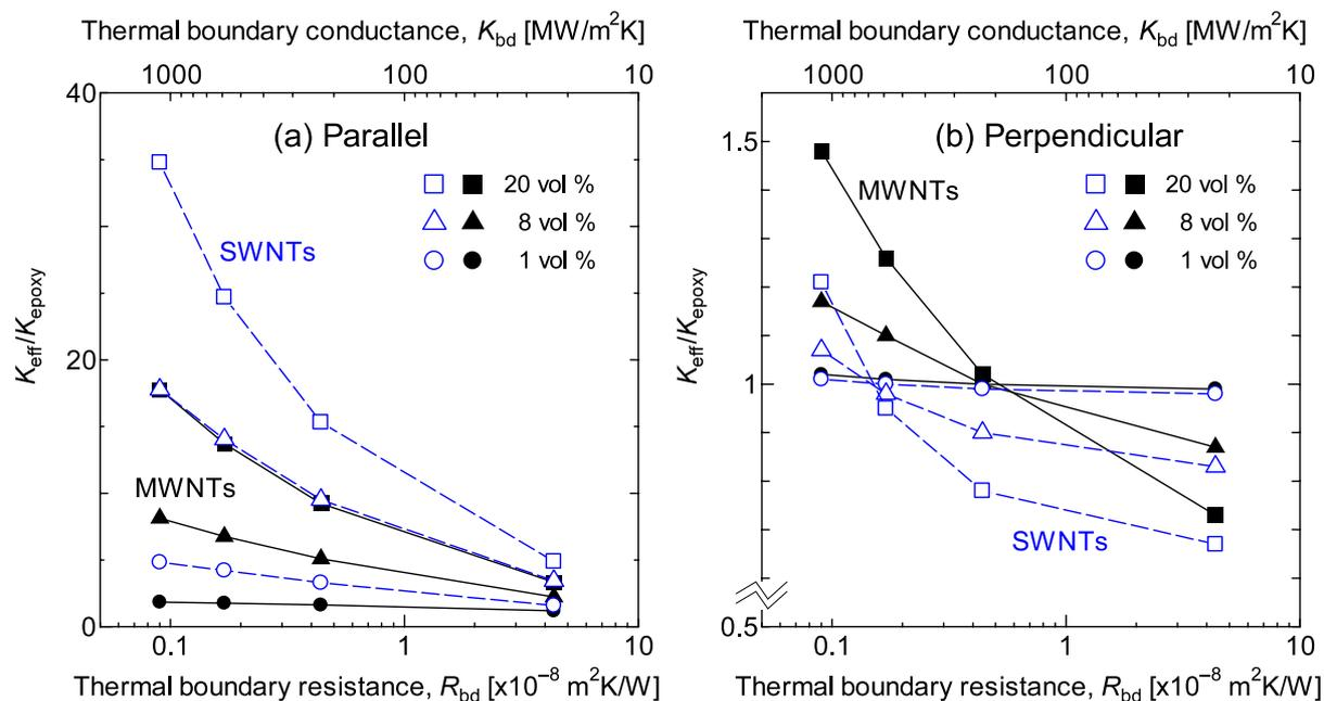
**Figure 6.** Comparison of effective thermal conductivity of MWNT-epoxy (solid dots) and SWNT-epoxy (open dots) composites with CNTs oriented (a) parallel and (b) perpendicular to the heat flux with the inter-CNT contact as a function of thermal boundary resistance with different volume fraction of CNTs.
