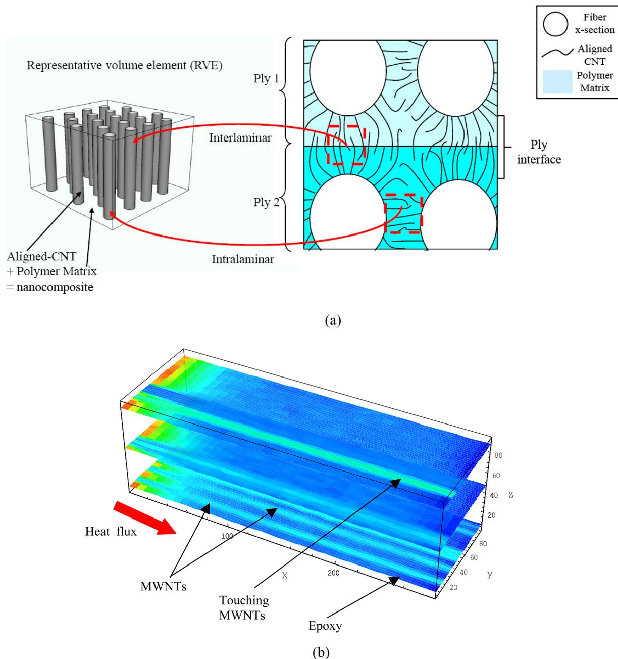
**Figure 1.** (a) Schematic drawing of three-phase CNT-reinforced composites, and aligned CNTs in a polymer as a representative volume element and (b) heat distribution of the MWNT-epoxy composite at 20 vol% of the MWNTs parallel to the heat flux at different  $z$  positions of the  $288 \times 96 \times 96$  grid epoxy cell. The cell is discretized into grid units for temperature evaluation.
