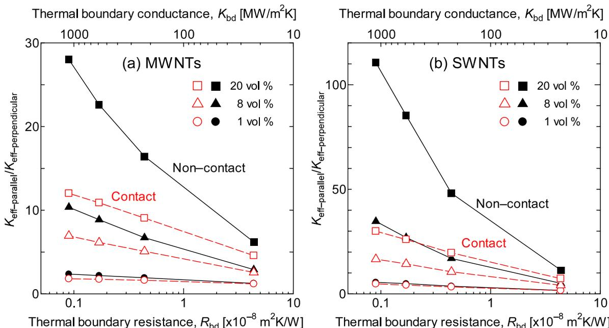
**Figure 4.** Effective thermal conductivity ratio ( $K_{\text{eff-parallel}}/K_{\text{eff-perpendicular}}$ ) of (a) MWNT- and (b) SWNT-epoxy composites without (solid dots) and with (open dots) the inter-CNT contact effects as a function of thermal boundary resistance with different volume fraction of CNTs.
