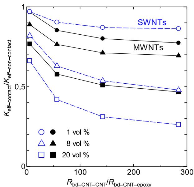
**Figure 7.** Effect of the relative conductance ratio ( $R_{bd-CNT-CNT}/R_{bd-CNT-epoxy}$ ) on the effective thermal conductivity of a composite when the inter CNT contact resistance is taken into account for MWNT (solid dots) and SWNT (open dots) epoxy composites having the CNT axis parallel to the heat flux direction.
