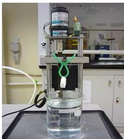
Figure 1 The setting of water absorption test
