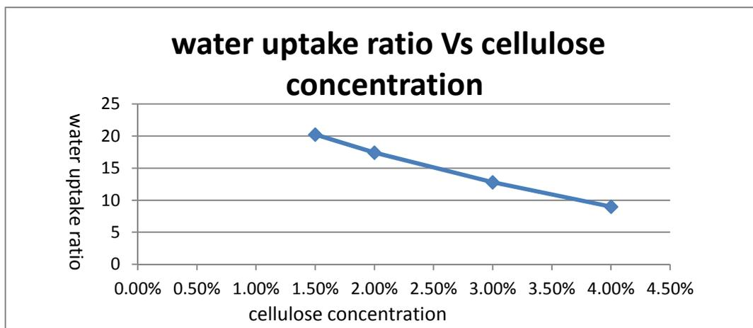
Figure 2 The water uptake ratio change with cellulose concentration
