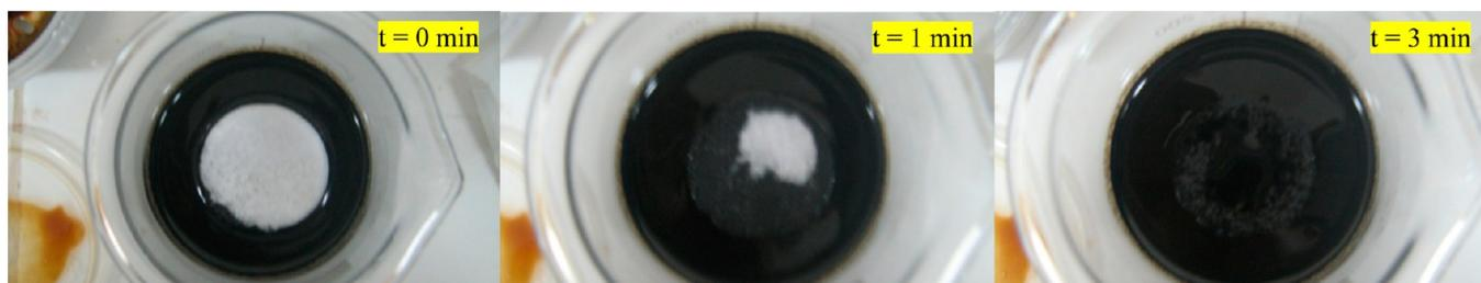
**Figure 3.** First minutes of the crude oil absorption process of the coated aerogel.
