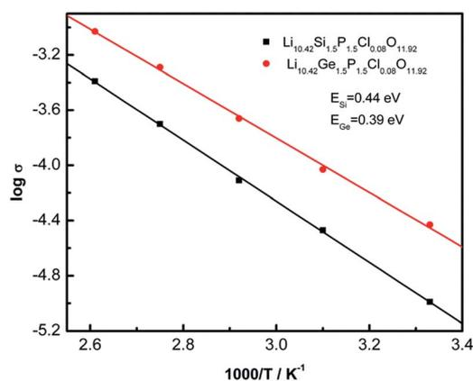
Fig. 2 Arrhenius plots of  $\text{Li}_{10.42}\text{Si}/\text{Ge}_{1.5}\text{P}_{1.5}\text{Cl}_{0.08}\text{O}_{11.92}$  in the range between  $27^\circ\text{C}$  and  $110^\circ\text{C}$ .
