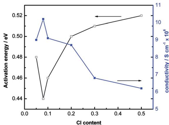
Fig. 4 The plots of room-temperature conductivity and activation energy versus Cl content.
