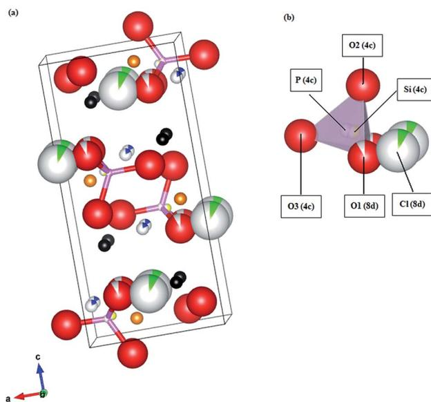
Fig. 7 (a) Ball and stick drawing of unit cell of  $\text{Li}_{10}\text{Si}_{1.5}\text{P}_{1.5}\text{Cl}_{0.5}\text{O}_{11.5}$ . (b) Enlarged view of the selected P/SiO/Cl<sub>4</sub> polyhedra. Li1 ions: black spheres, Li2 ions: orange spheres, Li3 ions: blue spheres, P ions: pink spheres, Si ions: yellow spheres, O ions: red spheres, Cl ions: green spheres.
