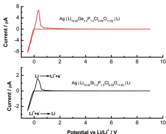
Fig. 5 The current-potential curves of  $\text{Li}_{10.42}\text{Si}/\text{Ge}_{1.5}\text{P}_{1.5}\text{Cl}_{0.08}\text{O}_{11.92}$ .
