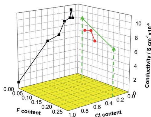
Fig. 3 Effect of halide substitution on the room-temperature conductivity of  $\text{Li}_{10.5-x}\text{Si}_{1.5}\text{P}_{1.5}\text{Cl}/\text{F}_x\text{O}_{12-x}$  ( $0.05 \leq x \leq 1.0$ ).
