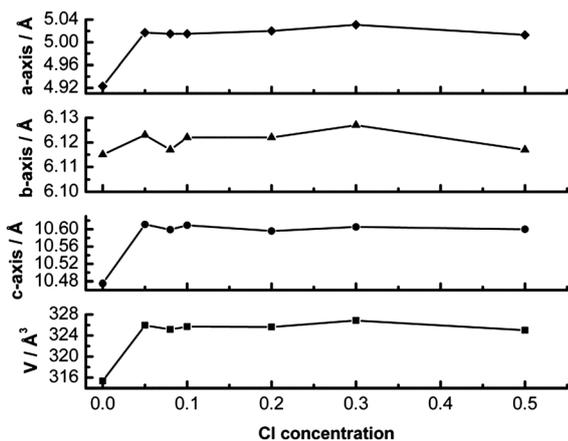
Fig. 6 The lattice constants and volume of unit cell of pure  $\text{Li}_3\text{PO}_4$  and Cl-substituted  $\text{Li}_{10.5-x}\text{Si}_{1.5}\text{P}_{1.5}\text{Cl}_x\text{O}_{12-x}$  solid solutions.
