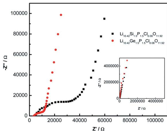
Fig. 1 Typical Nyquist plots of  $\text{Li}_{10.42}\text{Si}_{1.5}\text{P}_{1.5}\text{Cl}_{0.08}\text{O}_{11.92}$  (square symbol) and  $\text{Li}_{10.42}\text{Ge}_{1.5}\text{P}_{1.5}\text{Cl}_{0.08}\text{O}_{11.92}$  (circle symbol) measured at  $27^\circ\text{C}$ .
