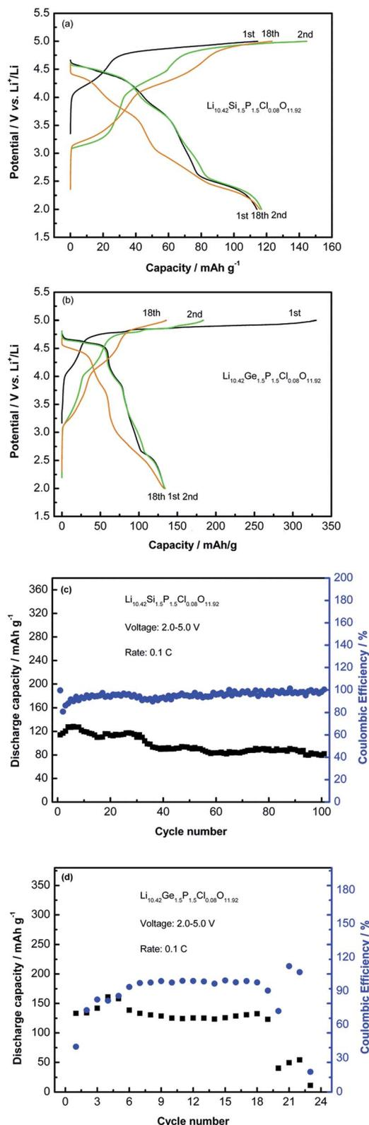
Fig. 9 (a) The charge–discharge curves of  $\text{Li}_{10.42}\text{Si}_{1.5}\text{P}_{1.5}\text{Cl}_{0.08}\text{O}_{11.92}$  and (b)  $\text{Li}_{10.42}\text{Ge}_{1.5}\text{P}_{1.5}\text{Cl}_{0.08}\text{O}_{11.92}$  cells at 0.1 C rate. (c) Cycle performance of  $\text{Li}_{10.42}\text{Si}_{1.5}\text{P}_{1.5}\text{Cl}_{0.08}\text{O}_{11.92}$  cells. (d) Cycle performance of  $\text{Li}_{10.42}\text{Ge}_{1.5}\text{P}_{1.5}\text{Cl}_{0.08}\text{O}_{11.92}$  cells.
